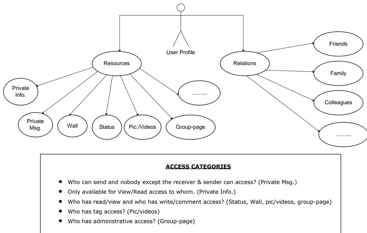
**Figure 3.1.** Basic structure of OSN user profile.
